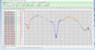
The product will be irradiated with a special developed Halogen lamp. The resulting diffuse reflection (the diffuse reflection contains the necessary information of the constituents) is transmitted via a fibre optic to the spectrometer. The spectrometer split the spectra in 256 support points.
